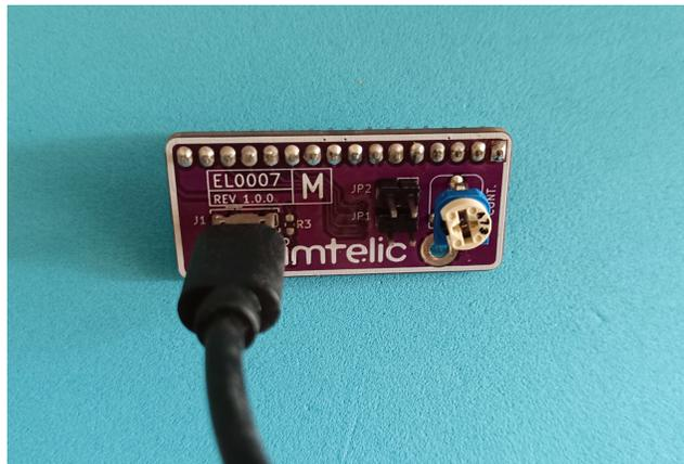
2. Connect the HD44780-based LCD to this module. This module is compatible with  $16 \times 2$  (1602),  $16 \times 4$  (1604) and  $20 \times 4$  (2004) character LCDs. Change the JP1 and JP2 jumpers according to the LCD type (see page 2).
