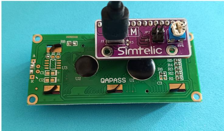
3. Connect the USB cable to the computer or SBC. In the default configuration, the LCD's backlight should be on and the display should show blank or white boxes.
