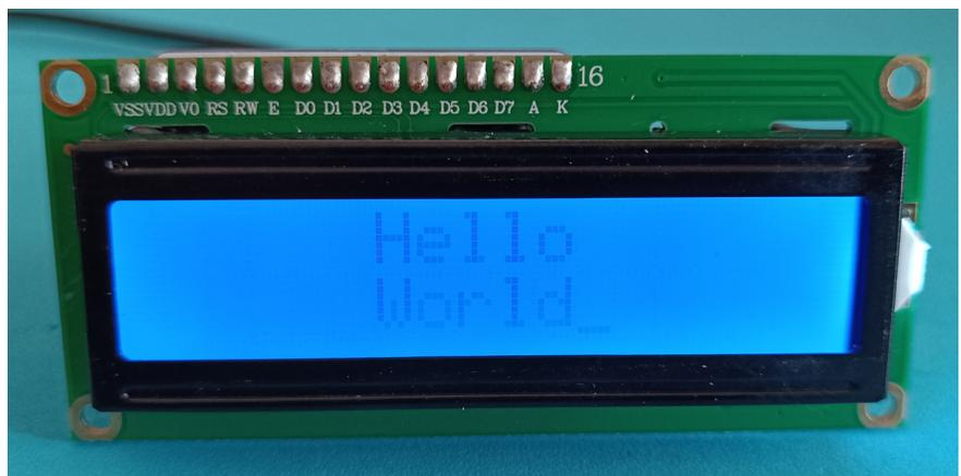
Correctly adjusted contrast leads to text on a clear background.
