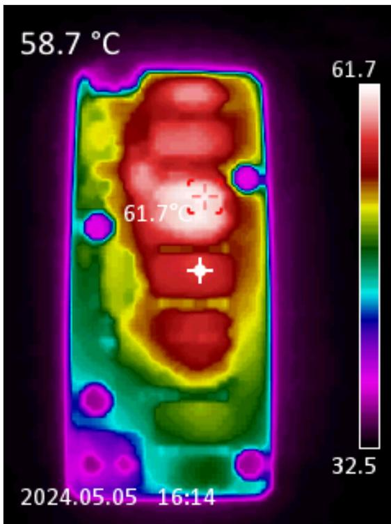
The test setup used to obtain these results involved attaching eight 24V automotive-grade relays into terminals J302 and J305 for 8 continuous hours.
